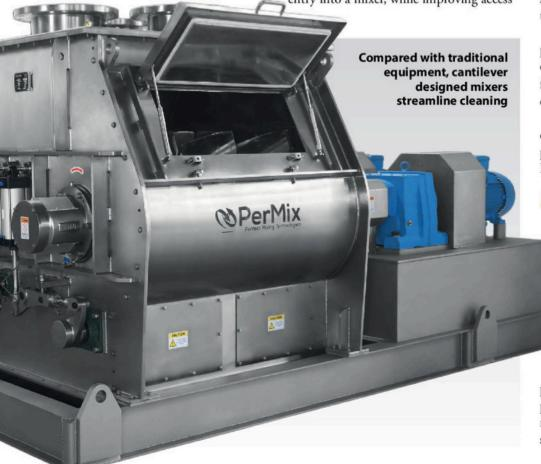
"The discharge valve is offset at a 15° angle, so it reduces the residue left in the mixer from an average of 2-3% to just 1%. With agitation style rotation, the powders create a slope inside the mixer that increases the total discharge," explains Paul.
