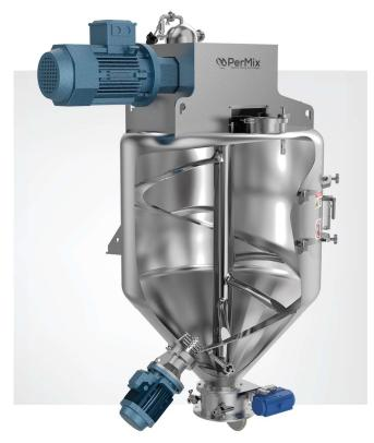
A side mounted access door is included for most of the models for inspection and cleaning purpose, and it is designed to be flush-fitting without creating blind areas for mixing and cleaning. At the bottom of the cone, there is a flush-fitting plug valve (manually or pneumatically operated) for product discharge.
