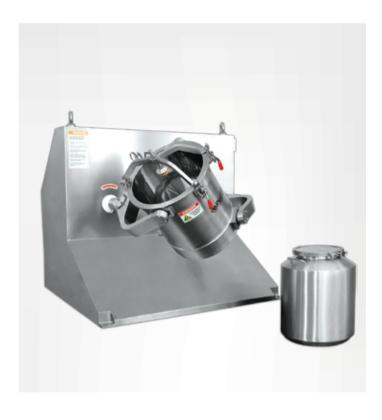
The PerMix PTU series 3D Mixer or Multi Direction Powder Mixer is used for homogeneous mixing of powdery substances with different specific weights and particle sizes. Producing dry-to-wet and wet-to-wet mixtures is also possible. The production process is hygienic and dust-free because the product is mixed in independent containers of variable sizes.
